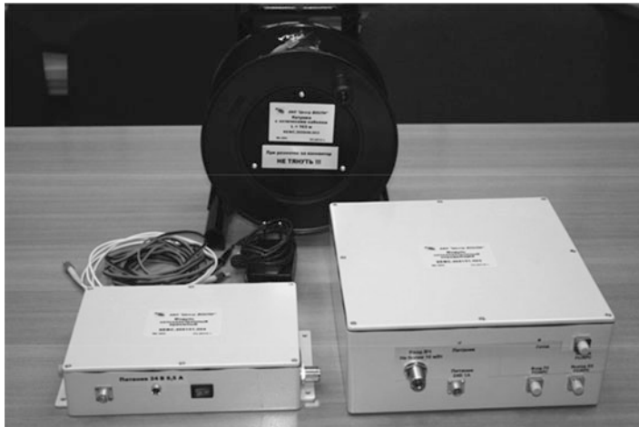
Fig. 11.40 Photo of stand units: optical receiver unit; optical transmitter unit with delay line; optic fiber coil (tripod with horn antenna is not shown) [1]
