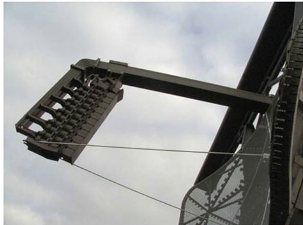
Fig. 4.16 An example of arrangement of twelve horn radiators on the antenna of the ASR 910 radar, which produces cosecant squared directivity pattern with layered beam
