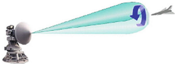
Fig. 4.29 During conical scanning, the radar tracks the conical diagram around the central axis
