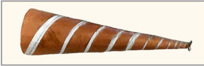
Fig. 4.154 Model of a log-spiral antenna
