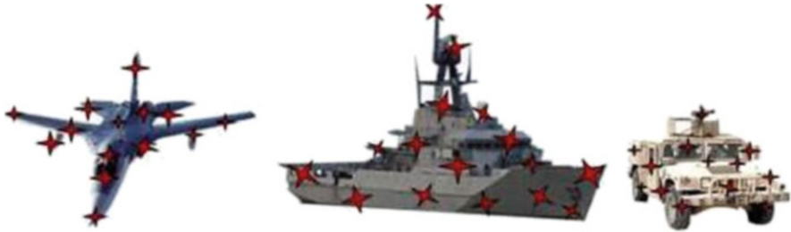
Fig. 1.14 Representation of a target as a combination of local reflection areas
