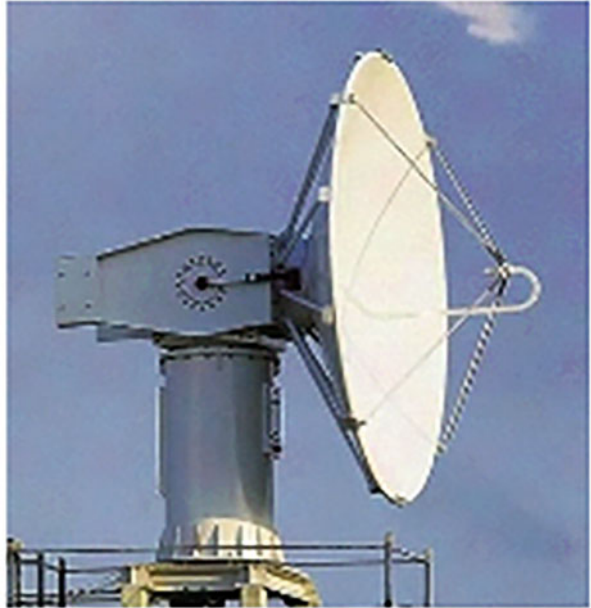
Fig. 4.7 Dish antenna of the Gematronc weather radar
