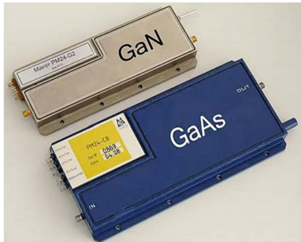
Fig. 6.23 Comparison between dimensions of amplifiers PM24-C8 (GaAs) and PM24-G2 (GaN)
