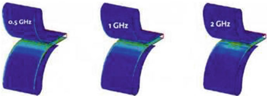
Fig. 4.64 Distribution of electrical power over radiating element
