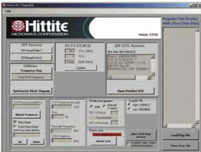
Fig. 8.119 GUI window for PLL synthesizer parameter control
