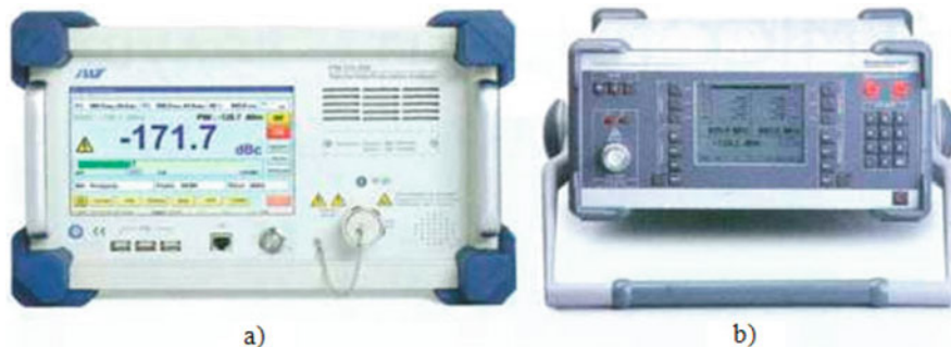
Fig. 10.85 Laboratory PIM-analyzers: (a) of S1L series made by AWT Global Company; (b) of Portable Type series made by Rosenberger Company;
